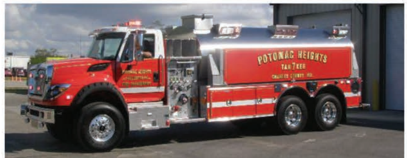
2013 Pierce Tanker 3500 Gallons/1000GPM
